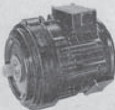
Chief source of electric power in TSR.2 is a pair of solid-state alternators, each of which is driven by a main engine through a Plessey constant-speed drive. The alternator is by Rotax, and has a rating of 30-75kVA.
